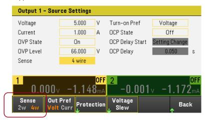
Figure 2. E36200 set 2-wire or 4-wire sensing for output 1 in just one click
